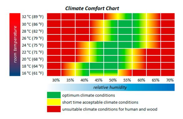
Maintaining the perfect Indoor climate through temperature and humidity control is not only important for our health and well being, but also for the longevity and performance of your Admonter Natural Floor and Wood Panels.
