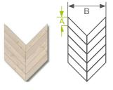
PATTERN WIDTHS FORMAT 45° 15 x 120 x 500 mm
